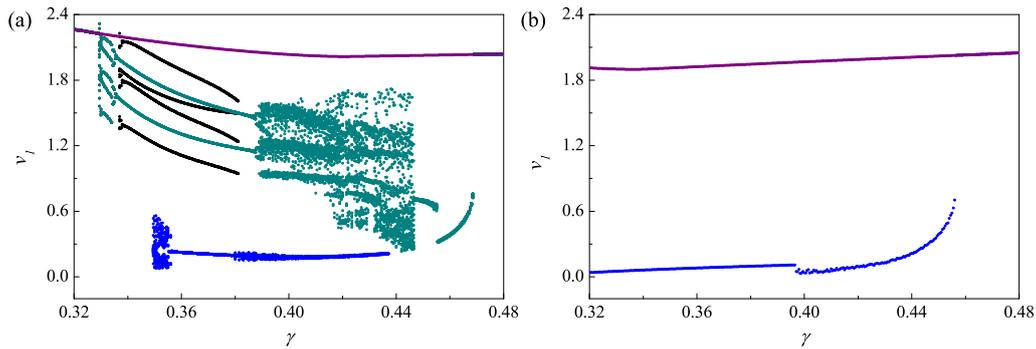
Figure 3: Bifurcation diagrams for the capsule system constructed for varying mass ratio  $\gamma$ , (a) without control ( $k_p = 0$ ) and (b) with control ( $k_p = -0.2$ ), calculated for  $\beta = 3$ ,  $\xi = 0.05$ ,  $\delta = 0.02$ ,  $\alpha = 1.6$ ,  $\omega = 1.1$ , and  $v_s = 0.1$ .
