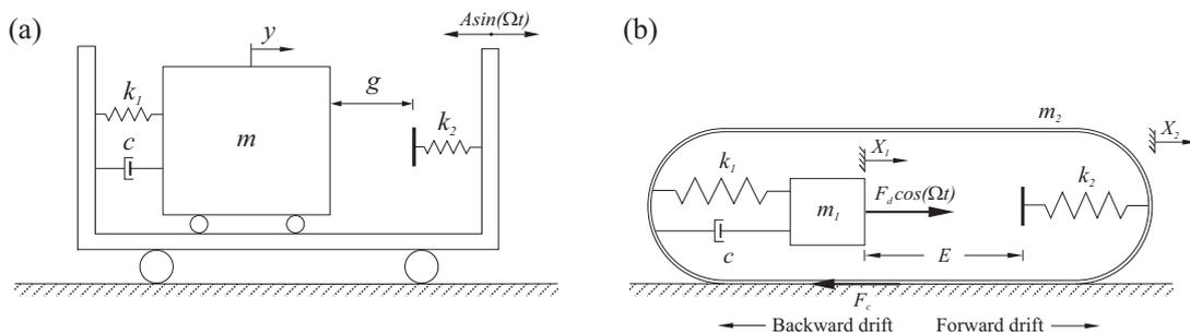
Figure 1: Physical models of (a) the impact oscillator and (b) the vibro-impact capsule system.
