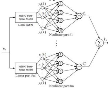
Fig. 2 Reduced-order model for aerodynamic systems
