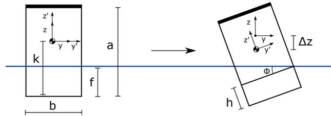
Figure 1: Geometry of a floating rectangular body in both tilted and upright positions with depth  $\ell$  into the page. Planar motion degrees of freedom are assumed where rotation  $\phi$  and vertical translation  $z$  give non-trivial equilibrium solutions.
