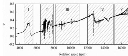
Fig.3 Bifurcation of the vertical displacement at Node 8.
