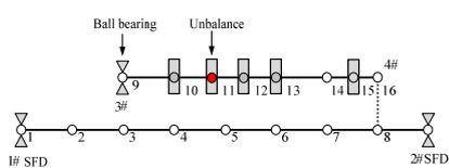
Fig.1 Computational model of the original system
