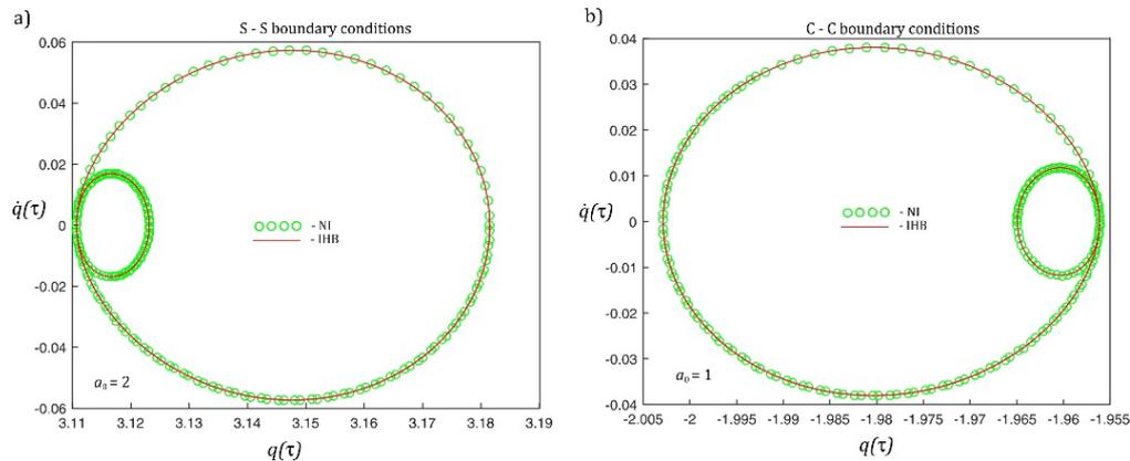
**Fig. 2** Periodic behavior of FG nanobeam obtained from IHB method, a) S-S and b) C-C boundary conditions.
