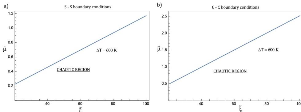
**Fig. 3** Bifurcation curves for FG nanobeam obtained from Melnikov function, a) S-S and b) C-C boundary conditions.
