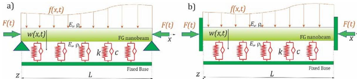
**Fig. 1** The FG nanobeam embedded in a viscoelastic medium, a) simply-supported and b) clamped-clamped nanobeam.
