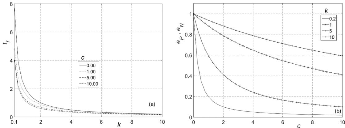
Fig. 2. Effect of parameters  $k$  and  $c$  on (a) duration of contact phase and (b) restitution coefficients.
