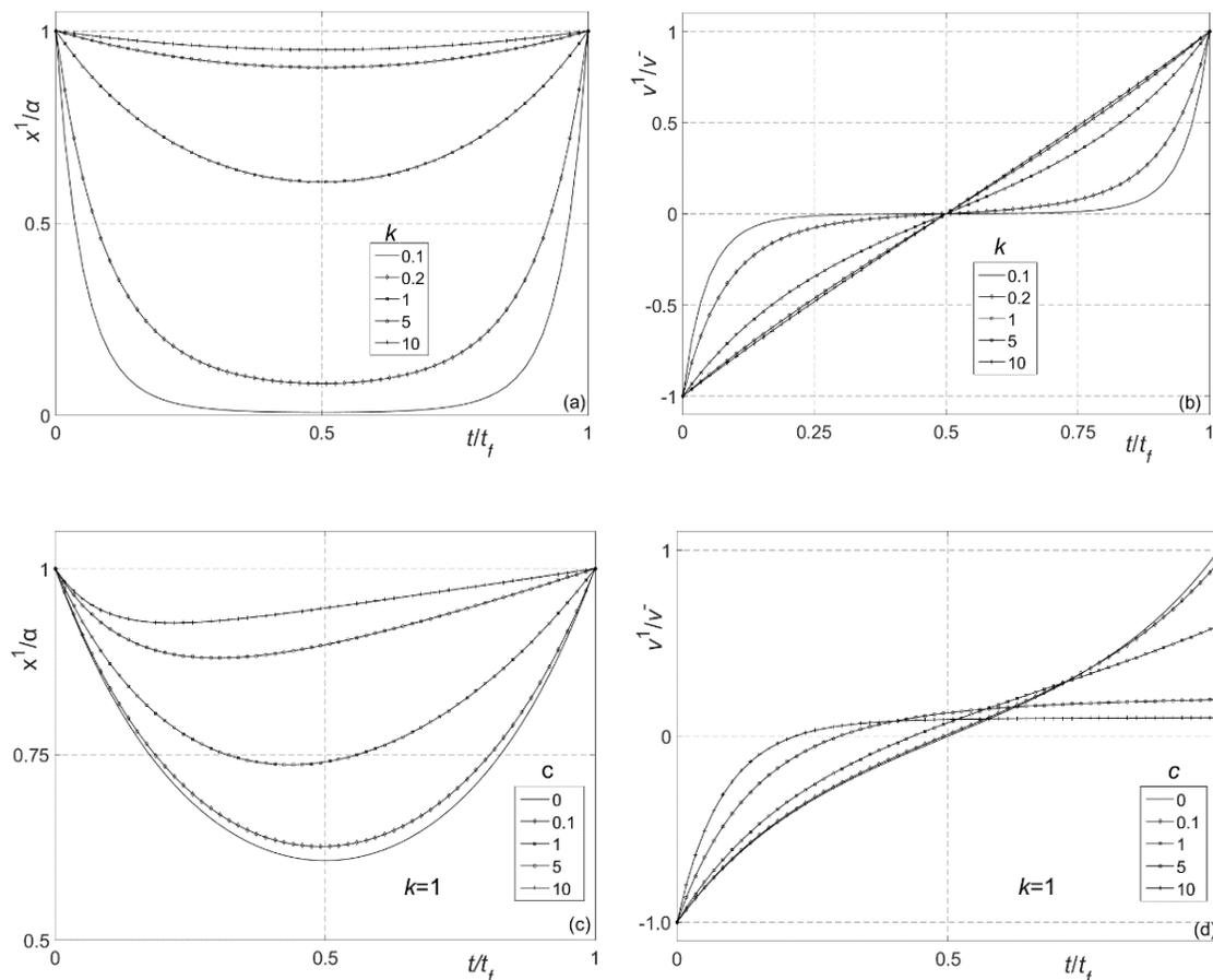
**Fig. 1.** Effect of the boundary forcing parameter  $k$  on the figurative particle (a) displacement and (b) velocity normal to the wall, for  $c = 0$ . Effect of parameter  $c$  on the (c) displacement and (d) velocity normal to the wall, for  $k = 1$ .
