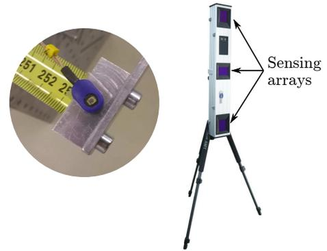
Figure 3: Acquisition equipment from CODAMOTION (marker and scanner).
