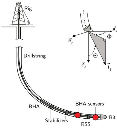
Figure 1: Schematic of a directional drilling system and inclination ( $\Theta$ ) and azimuth ( $\Phi$ ) angles of the bit measured from vector  $\vec{T}_1$  tangent to the borehole axis with respect to the earth's fixed frame.
