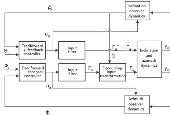
Figure 2: Closed-loop control strategy implemented to the directional drilling system.
