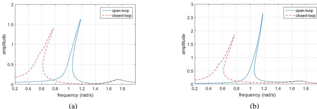
Figure 2. The amplitudes: open-loop marked with blue solid line and closed-loop marked with red dashed line (a),  $X_1$ , (b)  $X_2$
