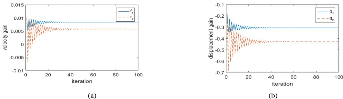
Figure 1. The feedback control gains at every iteration (a) velocity gains (b) displacement gains
