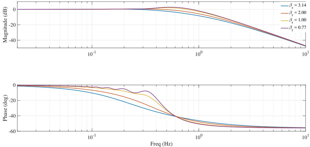
Figure 5: Frequency Response of GFrORE of order  $2\alpha = 2.5$  with  $\gamma = 0$  for different values of  $\beta_r$ .
