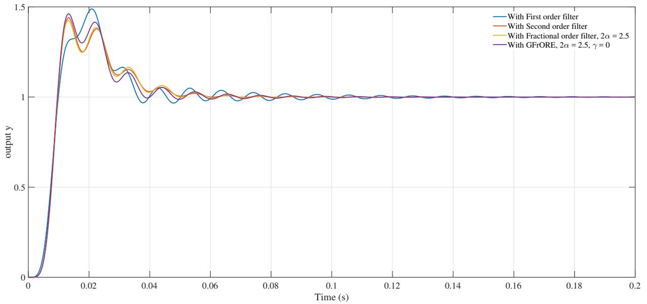
Figure 7: Step response for all controller configurations
