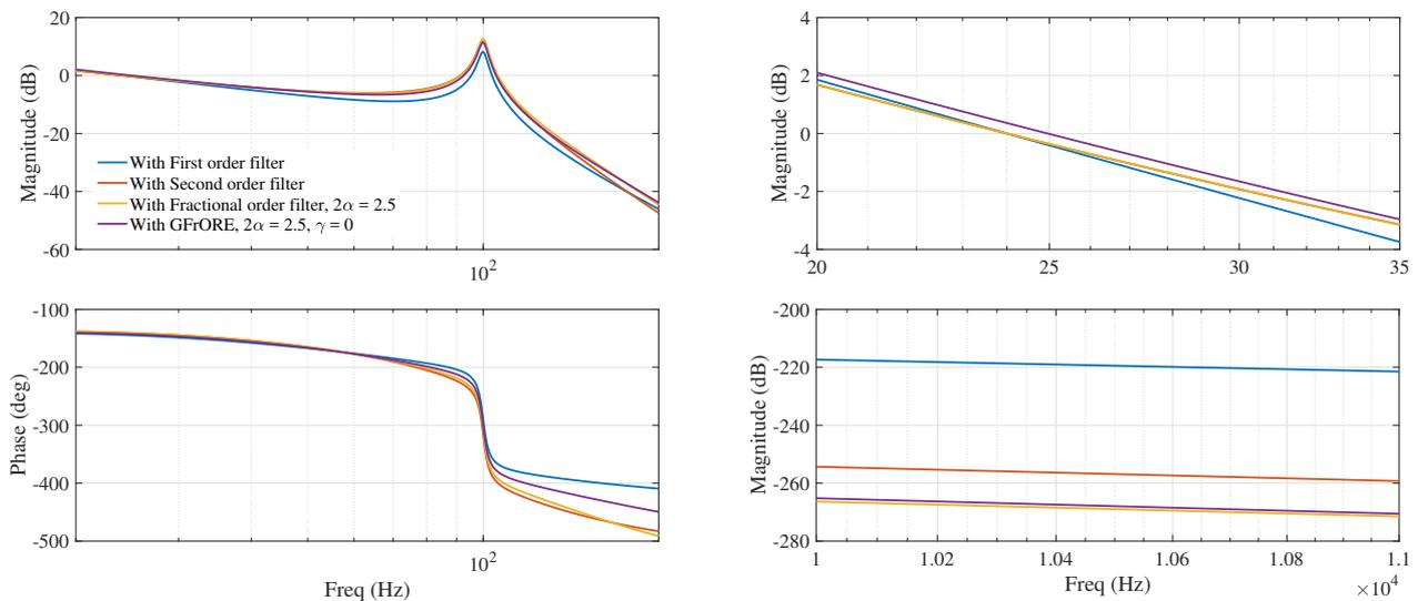
Figure 6: Open loop frequency response for all controller configurations provided. On the left is the overall open loop frequency response. On the right top is zoom in at the bandwidth and on the right bottom is at high frequencies where noise attenuation is necessary
