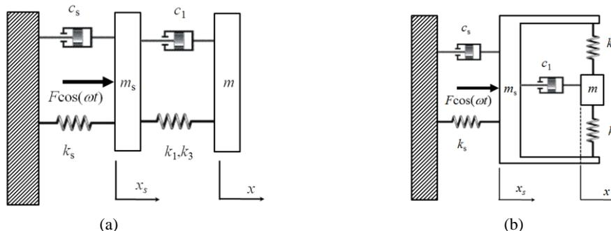
Figure 1. (a) Model of the system under study and (b) its mechanical implementation.
