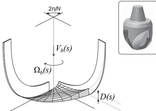
Figure 1: Downhole bit-rock interaction, from [2, 3].
