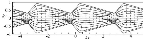
Figure 1: The curvilinear grids in the  $(x, y)$  plane that correspond to the Cartesian grids  $\xi = \text{const}$  and  $\eta = \text{const}$  in the mapped plane, showing the ‘terrain-following’ contours near the walls.
