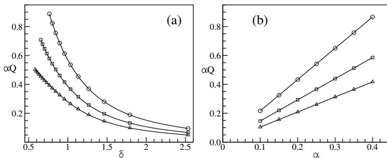
Figure 3: The pumping rate  $\alpha Q$  (for half channel width) (a) as a function of frequency (via the dimensionless Stokes layer thickness  $\delta = \sqrt{2\nu/\omega}/h_0$ ) for oscillation amplitude  $\alpha = 0.3$ ; (b) as a function of  $\alpha$  for  $\delta = 0.9247$ . Channel lengths:  $\circ$ ,  $N = 15$ ;  $\square$ ,  $N = 10$ ;  $\triangle$ ,  $N = 5$  (multiple of  $\lambda_s$ ).  $\epsilon_b = 1.0$ ,  $\beta = 0.3130$ .
