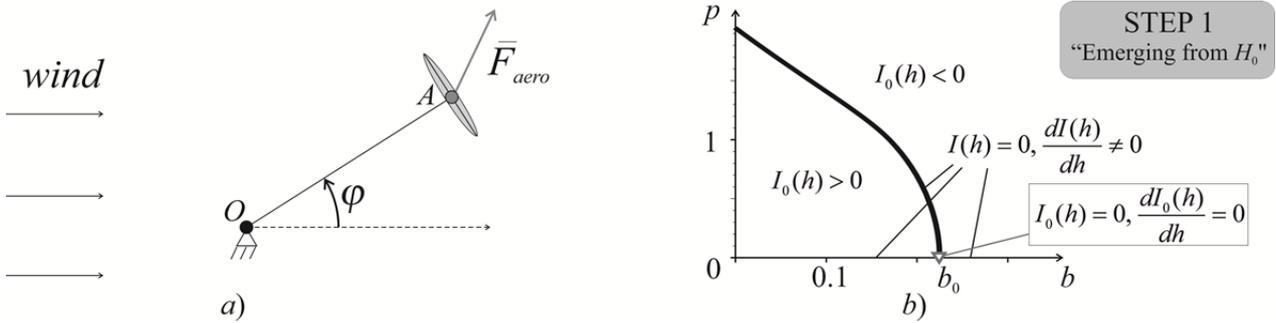
Fig. 1 a) An aerodynamic pendulum (top view); b) Bifurcation diagram of periodic trajectories emerging from trajectories of  $H_0$ .
