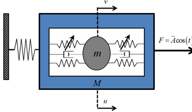
Figure 2-System scheme- linear oscillator as the primary system and internal particle with both linear and cubic attachments. The displacements of the primary mass and the impacting mass are denoted as  $u$  and  $v$ , respectively.
