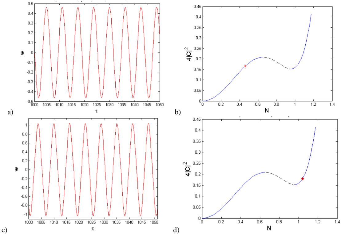
Figure 5-double periodic solution, corresponding to Figure 4(b):  $k = 4/3, \sigma = 5, \varepsilon = 0.05, A = 1.62$ ,
