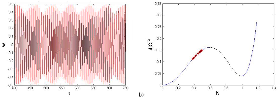
Figure 6- Quasi-periodic solution, corresponding to Figure 4(c):  $k = 4/3, \sigma = 5, \varepsilon = 0.05, A = 1.4, \beta = 5 \Rightarrow \lambda_{cr,H} = 0.268, \lambda_{cr,SN} = 0.577, \lambda = 0.1 < \lambda_{cr,H}$ . Initial conditions:  $u_0 = v_0 = 0, \dot{u}_0 = 0.5, \dot{v}_0 = 0$ .
