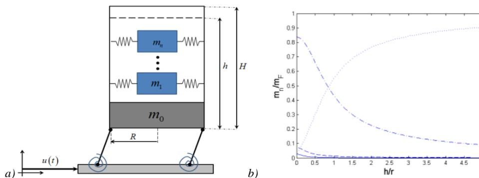
Figure 1-a) Scheme of multiple sloshing modes in partially-filled tank represented by a series of mass-spring systems; b) Ratios of the first three asymmetric sloshing modal masses and fixed mass  $m_0$  to the total fluid mass  $m_f$  for cylindrical vessel; dotted-line, dashed-dotted-line, dashed-line, solid-line, respectively.
