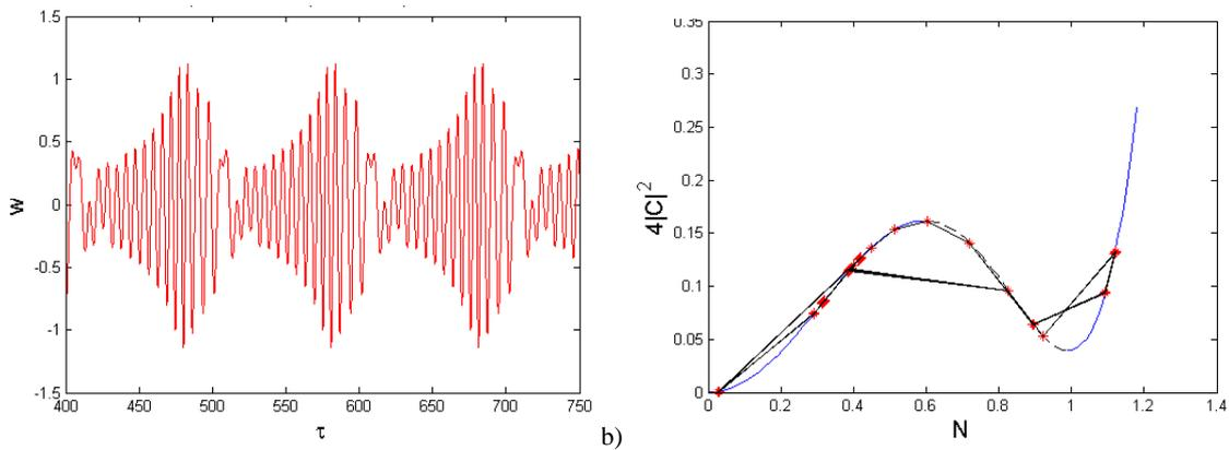
Figure 7- SMR regime:  $k = 4/3, \sigma = 0, \varepsilon = 0.05, \beta = 1, A = 0.3, \lambda = 0.2 \Rightarrow A > A_{cr,SMR} = 0.176$ . Initial conditions:  $u_0 = 0.29, v_0 = -0.5, \dot{u}_0 = 0.9, \dot{v}_0 = -0.15$ .
