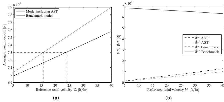
Figure 2: (a) Averaged value  $\hat{W}$  of the total weight-on-bit  $W$  and (b) averaged value of the cutting force  $\hat{W}^c$  and wearflat contact force  $\hat{W}^f$ , both as function of the prescribed top-drive axial velocity  $V_0$ , for  $\Omega_0 = 120$  rpm.
