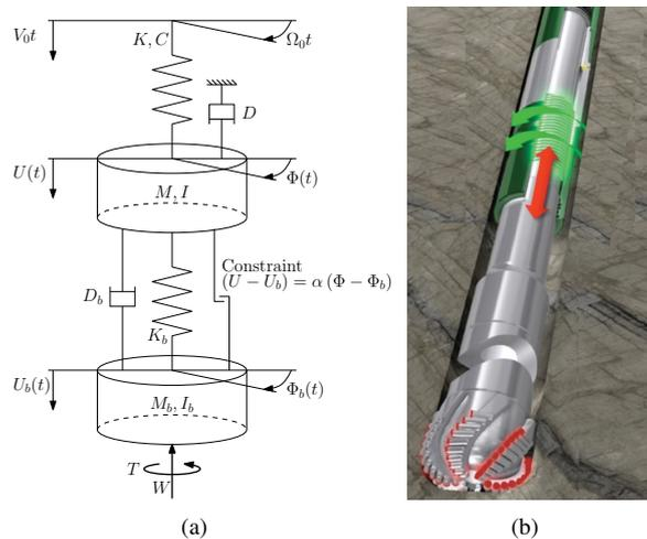
Figure 1: (a) Schematic model of a drill-string including anti-stall tool (AST). (b) Impression of the working principle of the AST [4].
