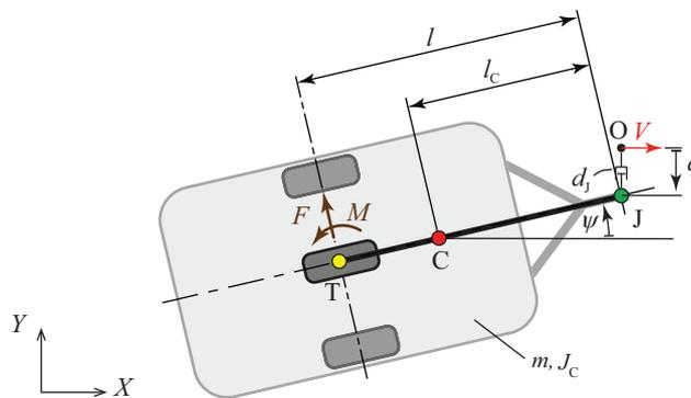
Figure 1: The in-plane single-track model of the towed trailer.
