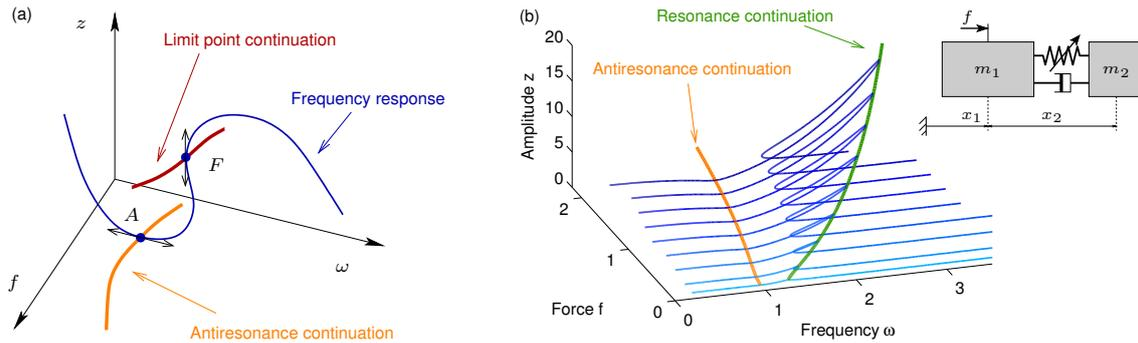
Figure 1: (a) Geometric illustration of limit point and antiresonance continuation; (b) nonlinear tuned mass damper and frequency response of the first harmonics of  $x_1$  for several value of the forcing  $f$  and antiresonance and resonance continuation.
