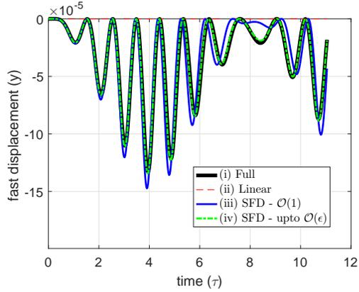
(b) Displacement (in m) at quarter length of beam in the axial direction (Fast y DOF).
