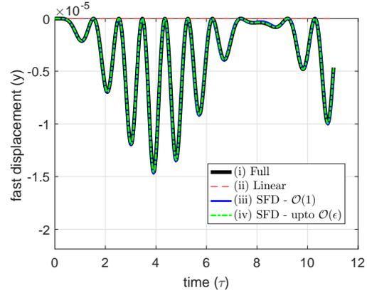
(b) Displacement at quarter length of beam in the axial direction ( Fast y DOF).
