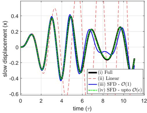
(a) Displacement at quarter length of beam in the transverse direction (Slow x DOF).
