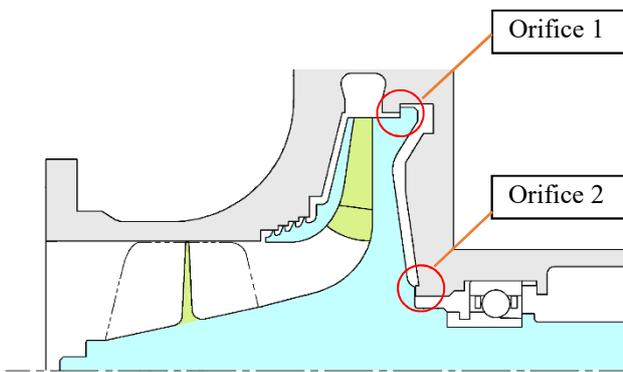
Fig.1 A cross section of rocket turbo pump
