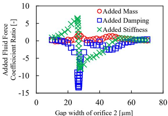
Fig.5 Calculated added fluid force coefficient ratio
