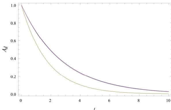
Fig.1. Amplitude-time function for the damping oscillator for preloading of: T=5 lb (blue line), T=7.5 lb (magenta line) and T=10lb (green line).
