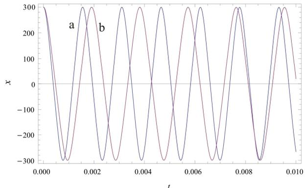
Fig.2. x-t diagrams for the damped system with various preloading: a) T=5 lb (blue line), b) T=7.5 lb (red line).
