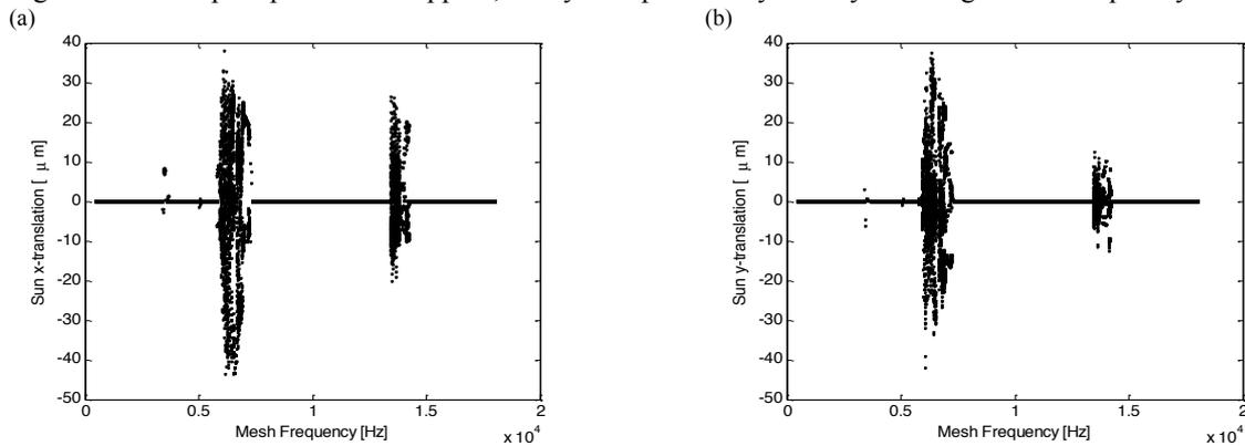
Fig. 2. Bifurcation diagram vs. mesh frequency for case 2 (a) Sun center x-translation [ $\mu\text{m}$ ], (b) Sun center y-translation [ $\mu\text{m}$ ]
