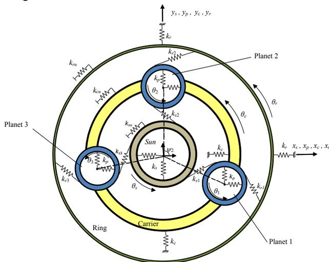
Fig. 1. Physical planar model of the single stage planetary gearbox
