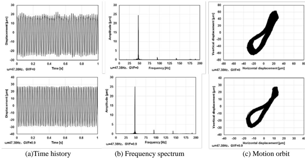
Figure 11 Rotor response with large imbalance at  $\omega=47.38\text{Hz}$ ,  $\text{GVF}=0$  and  $0.9$
