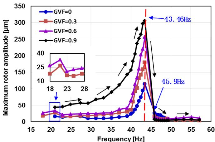
Figure 3 Amplitude-frequency curves under different GVF
