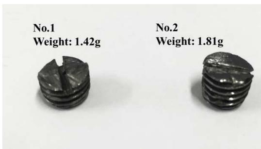
Figure 4 Bolts used to add imbalance
