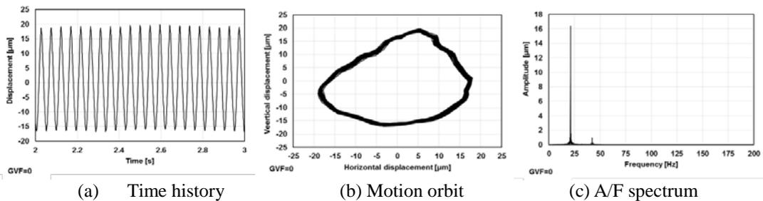
Figure 7 Dynamical response of rotor for pure oil at 21Hz
