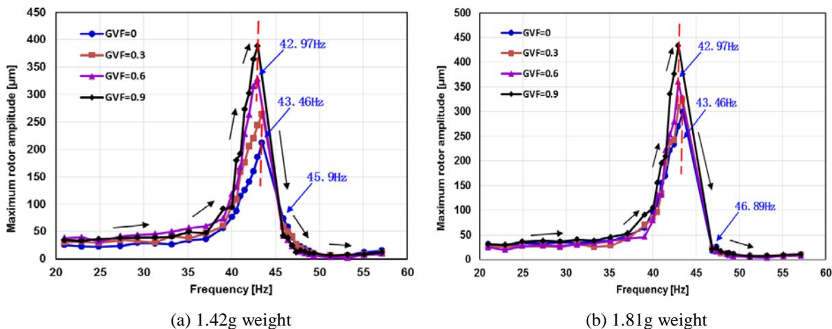
Figure 5 Amplitude-frequency curves under different GVFs at inlet
