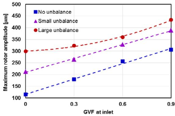
Fig.6 Maximum amplitude of rotor at different GVFs and imbalance
