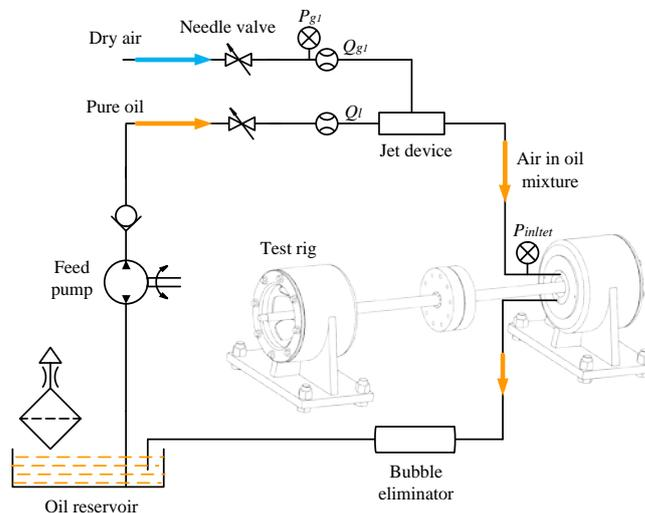
Figure 2 Squeeze film damper lubrication systems
