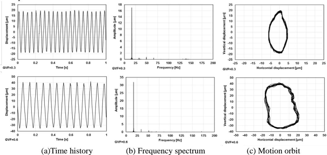
Figure 8 Rotor response at 18.13Hz, GVF=0.3 and 0.6
