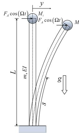
Figure 1: The scheme of the cantilever beam energy harvester with lumped mass on the free end.
