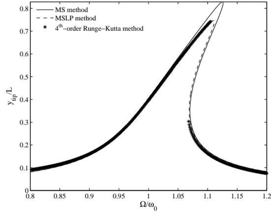
(a) Comparison of the first mode FRCs obtained by MS method, MSLP method and numerical simulation with parameters being  $\omega_0 = 7.4853\text{rad/s}$  and  $F_A = 0.004N$ .
