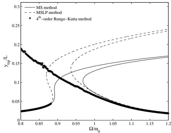
(c) Comparison of the third mode FRCs obtained by MS method, MSLP method and numerical simulation with forcing parameters being  $\omega_0 = 149.1810\text{rad/s}$  and  $F = 0.4N$ .
