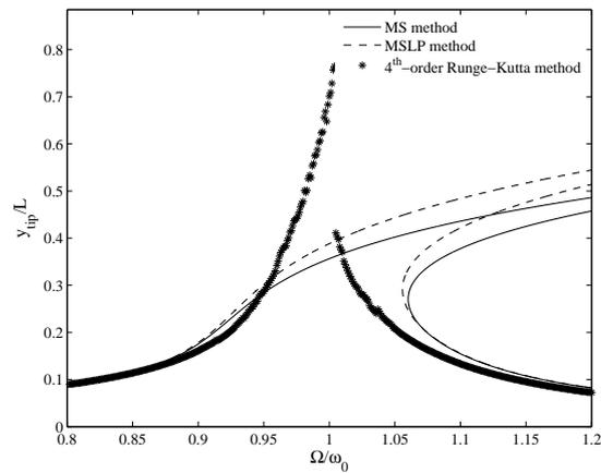
(b) Comparison of the second mode FRCs obtained by MS method, MSLP method and numerical simulation with parameters being  $\omega_0 = 52.7202\text{rad/s}$  and  $F = 0.2N$ .
