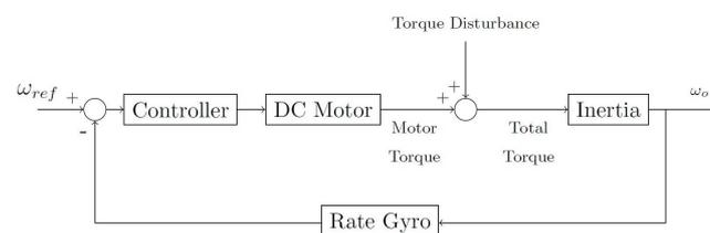
Figure 2: Block scheme of the controlled system
