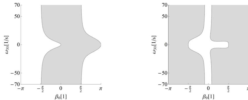
Figure 2: Conditions of the realisable stationary motions. Each point of the plane correspond to a stationary motion according to (2). Left panel: the shaded area shows the solutions which the ball does not fall from the rim. Right panel: the shaded area show the solutions which are stable. The numerical values of the parameters are the values of the standard basketball and basketball rim.
