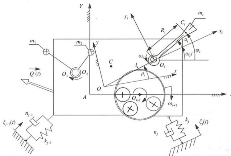
Fig. 14. Object with synchronous eliminators of vibrations
