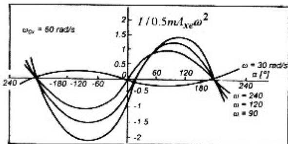
Fig.11. Vibratory force as a function of the ball position for  $\omega > \omega_0$  and  $\omega < \omega_0$
