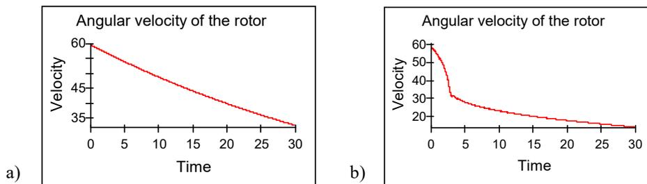
Fig. 9. Behaviour of the rotor without the moment  $T_m$
