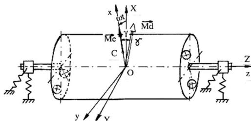
Fig. 12. Balancing in two planes
