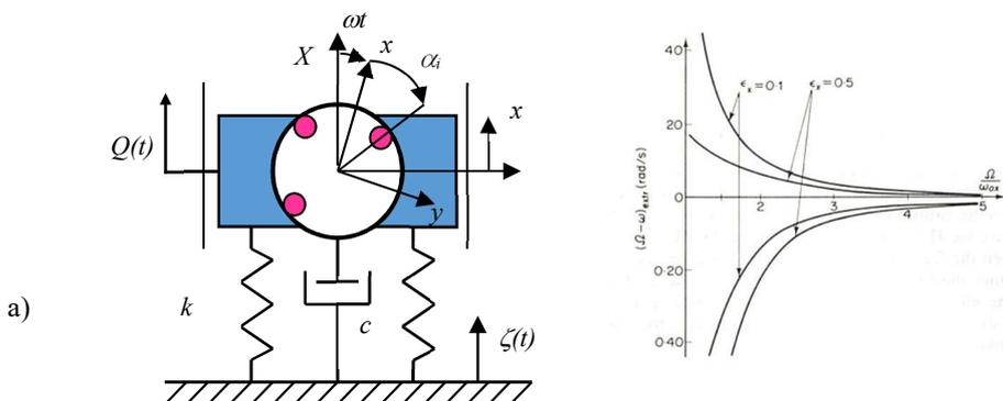
Fig. 13. Synchronous eliminator of vibration (a) and allowable frequency difference (b)  $\Delta\omega$  if  $c=0.05 \text{ kg/s}$ .
