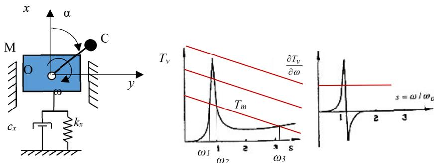
Fig.8. Unbalanced rotor and its dynamic characteristics
