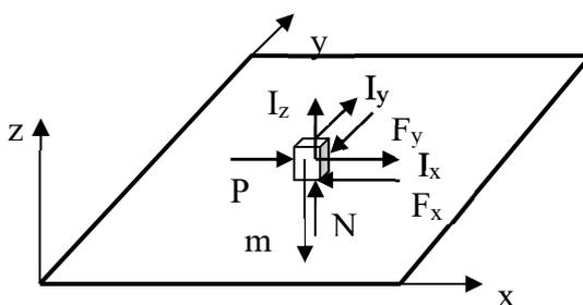
Fig.15. Block on vibrating plane
