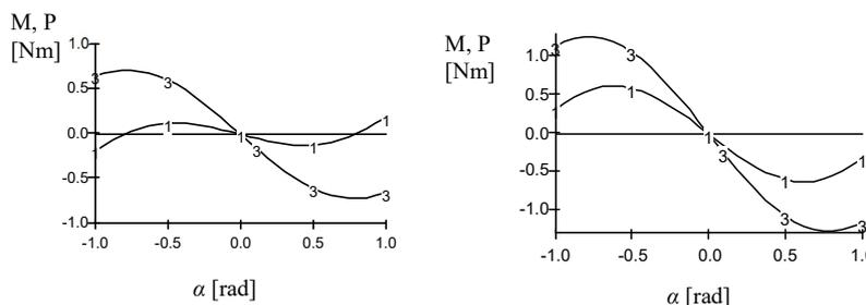
Fig.7. Total moment M (1) and vibratory moment P (3) if  $\Omega=150$  (a),  $200 \text{ rad/s}$  (b) and  $\beta=0$ ,  $\alpha_o=\pi$
