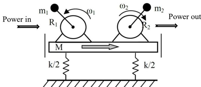
Fig. 4. Transmission of power between two rotors
