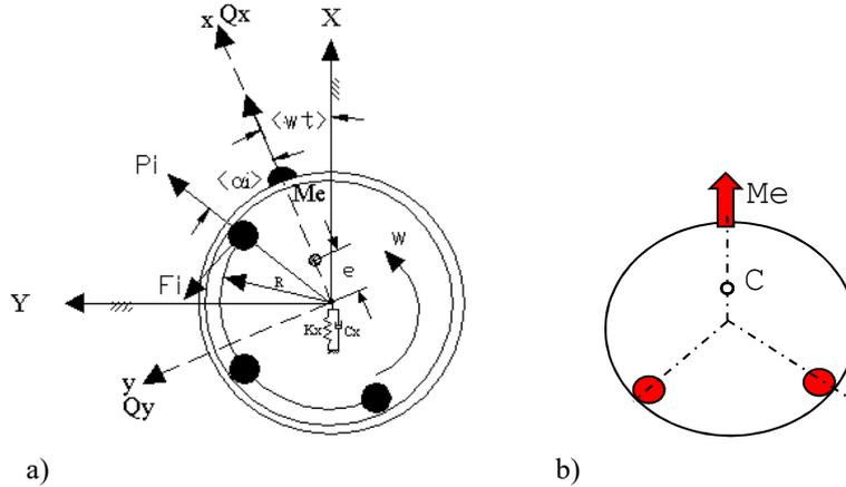
Fig.10. Unbalanced rotor (a) and the final position of the balls (b)
