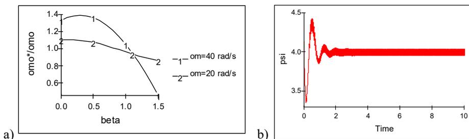
Fig.6. Change of natural frequency of the pendulum for lower position and vibration  $\psi(t)$  of the pendulum for upper position if  $A = 16 \text{ mm}$ ,  $\Omega=150 \text{ rad/s}$ ,  $\beta=30^\circ$
