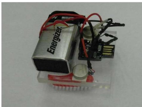
Fig.2. Vibratory robot with two disc motors
