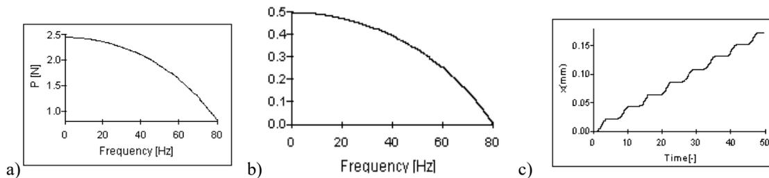
Fig. 15. Minimum force, equivalent coefficient of friction and the motion of the block (50 Hz) for  $m=0.5$  kg,  $\mu_0=0.5$ ,  $a_x=a_y=10$   $\mu\text{m}$
