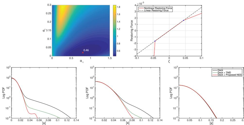
Figure 2: Top: grid search optimization with respect to  $\alpha_{-1}$  and  $\alpha_1$  (left) and the corresponding optimal restoring curve (right). Bottom: seat response PDF comparisons. No attachment (black), optimal TMD (green), and optimal proposed NES (red). See [1] for details.
