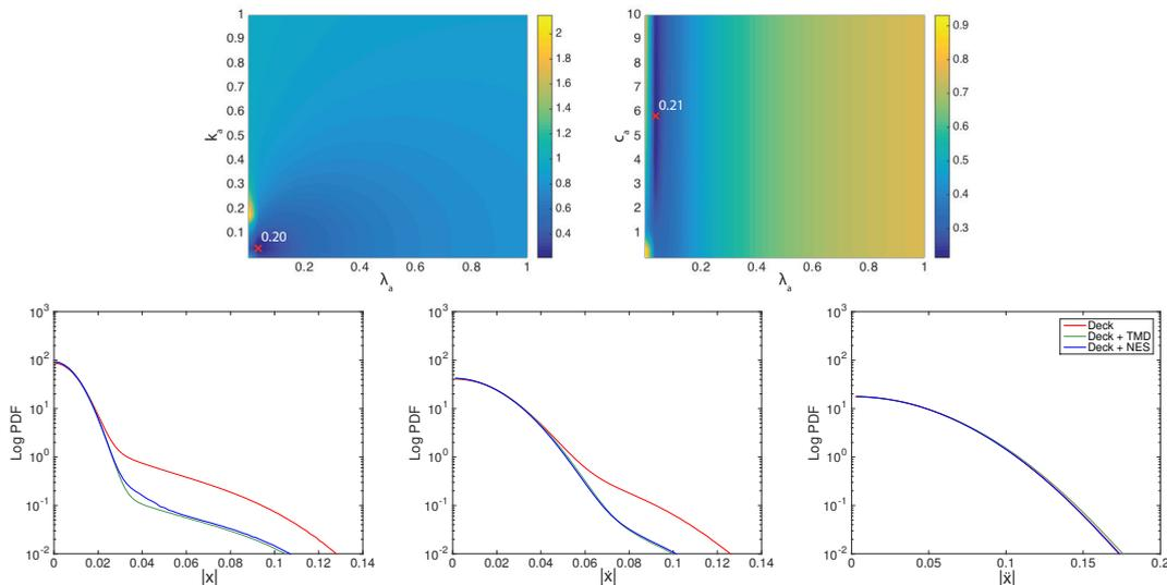
Figure 1: Top: grid search optimization of the suspended deck with tuned mass damper ( $c_a = 0$ , left) and nonlinear energy sink ( $k_a = 0$ , right). Bottom: seat response PDF comparisons. No attachment (red), optimal TMD (green), and optimal NES (blue).
