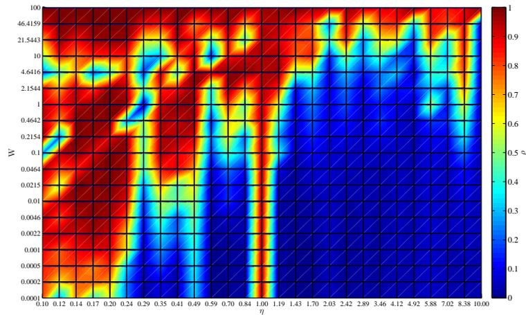
Figure 3: surface sample perception ratio  $\rho$  for varying  $\eta$  and  $W$ , and for  $\psi = 3.162$  (linear scale contour)
