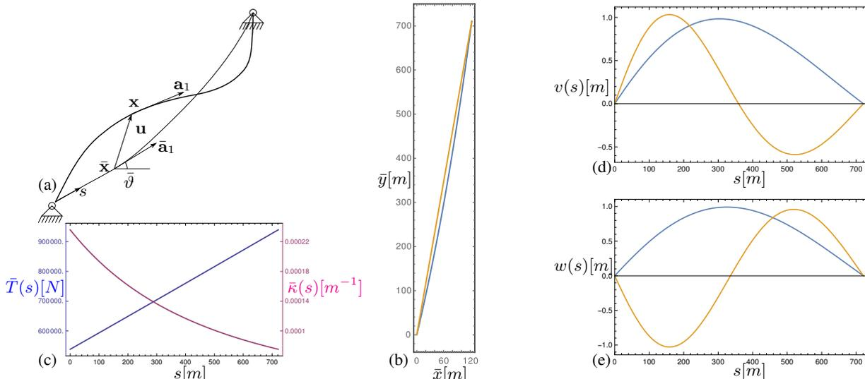
Figure 1: Stay-cable. (a) Static position  $\bar{x}$  and current position  $x$  of the axis line, with respective tangent vectors  $\bar{a}_1$  and  $a_1$ ; (b) Static configuration for the example (in blue), with inclined chord (in orange); (c) static pre-stress  $\bar{T}$  (in blue), and curvature  $\bar{\kappa}$  (in magenta) as function of  $s$ ; (d) in-plane modes: first (blue) and second (orange); (e) out-of-plane modes: first (blue) and second (orange).
