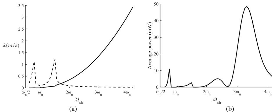
Fig 2. (a) Numerically computed velocity of the oscillator in Eq. (2). (b) Corresponding load power.
