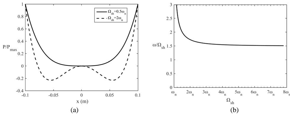
Fig 1. (a) Normalized potential energy of the conservative system corresponding to Eq. (2). Two values of  $\Omega$  are shown that result to single-well and double-well structure; (b) Frequency of torsional vibrations over the system's linear frequency. As the shaft speed increases, it approaches a fixed value of 1.5.
